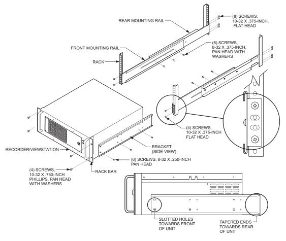
Figure 6. DX9100 Rack Mount Installation
